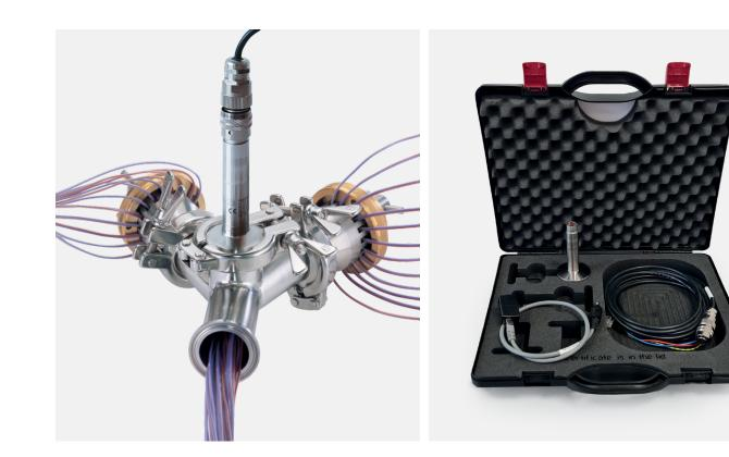
International and European norms (EN285, EN554, ISO-17665) for the validation of pharmaceutical, biotechnology and medical devices require the proof of saturated steam conditions in autoclaves. To achieve that a high accurate - temperature compensated -Pressure Transducer is needed.
