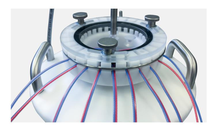
The Kaye Liquid Nitrogen (LN2) Comparator is a device specifically designed to address the calibration needs for extreme cold temperatures. With the ability to calibrate up to 48 Sensors at a time it addresses capacity and flexibility needs for thermal calibration at cryogenic temperatures.
