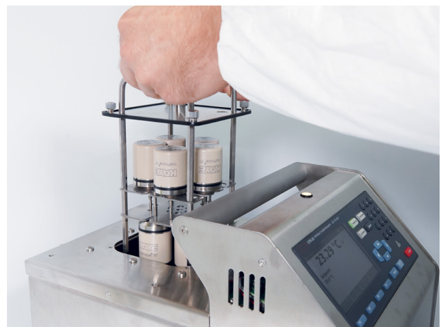
Picture 20: Kaye CTR-25 Calibration Bath with special insert for dataloggers
