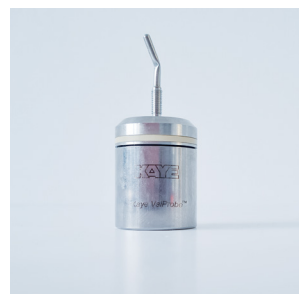
Picture 25: Mechanically damaged probe tip of the data logger
