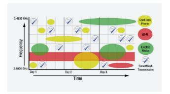
In addition the mesh protocol permits the system to learn about the RF environment and dynamically adjust the network parameters to best fit the current situation. The network provides an accurate time reference for the whole network, ensuring all loggers and the base station are time synchronized correctly. Each data sample is timestamped with this network time. Coexistence with Other RF Systems
