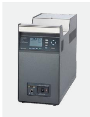
LTR-90 ( -90^{\circ}\text{C} to 150^{\circ}\text{C} ) up to 15 Thermocouples
