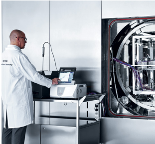
Picture 21: Professional Kaye thermocouple implementation on an autoclave
