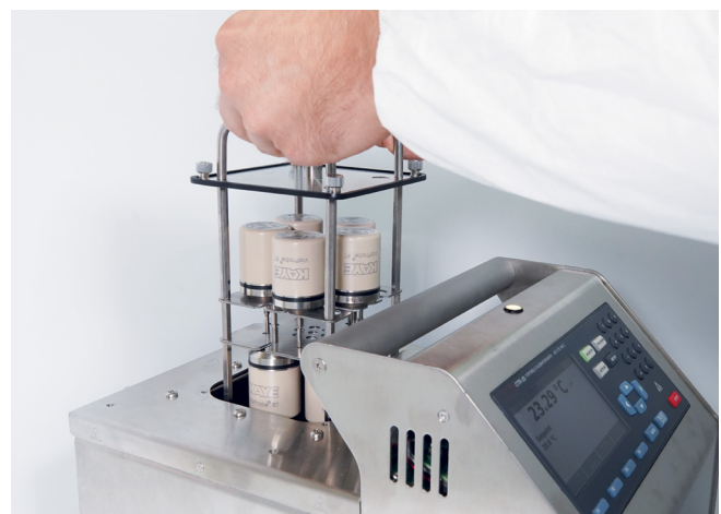
Picture 20: Kaye CTR-25 Calibration Bath with special insert for dataloggers
