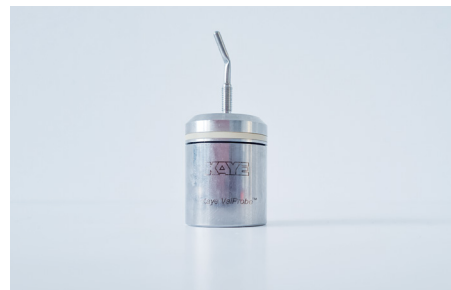
Picture 25: Mechanically damaged probe tip of the data logger
