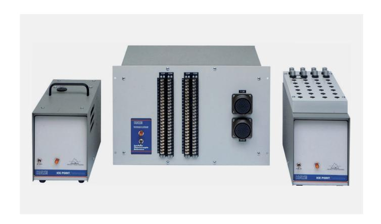
The K170 Ice Point Reference performs ice point referencing for up to 75 thermocouples. The user wires external thermocouples to the unit's input terminals which are in turn connected to matching internal TCs that terminate to copper at the temperature of a thermoelectrically produced ice-water mixture. Thermocouple-grade copper wire is taken from ice to MIL style connectors for output. Individual pass-through shield connections can also be provided.
