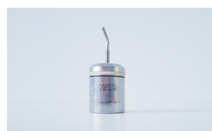
Picture 25: Mechanically damaged probe tip of the data logger
