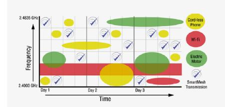
Frequency hopping ensures reliable transmission
