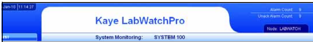
Figure 3: Header with Time, Date, User Name, Current Screen, Alarms and Node
